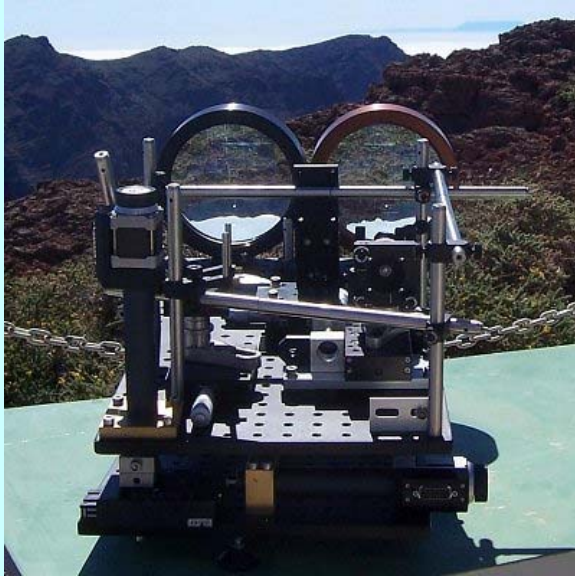
Single photon transmitter optics module (Alice) in La Palma aligned towards Tenerife (visible in the upper right corner).
