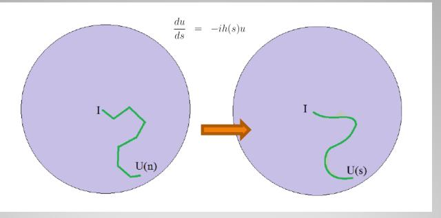
The left side shows a discrete path induced by a series of gates. The right side shows a curve induced by a tangent operator h(s).
