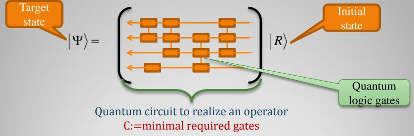
• Complexity for one operator is defined as the minimal required gates when we realized this operator by quantum circuits.
